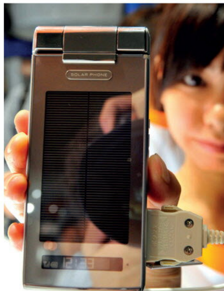
Mobile phone with an integrated solar panel to provide battery power
